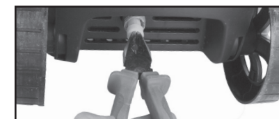
Pulling the filter out of the water inlet fitting, Fig. 14
